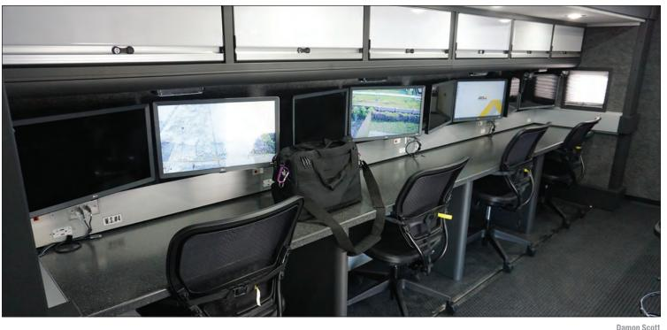
The interior of the vehicle has state-of-the-art features, such as LCD touch screens with custom graphics for local control and monitoring systems.
